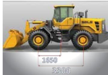
Weichai engine (two-stage) is adopted to realize large torque, strong power, low oil consumption, high quality and low emission. Dalian Deutz BF6M series engines is optional.
