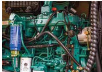
It is equipped with 93-type sand and dust filter with primary filtration accuracy up to over 93%; it is safe and reliable, and more suitable to sandy and dusty working condition.
